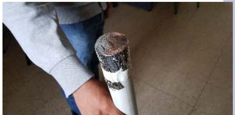
Figure 9. Aluminum paper being placed in the other extreme of the pipe.
