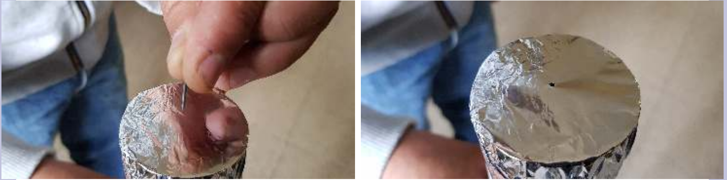
Figure 10. The tiny hole through which light goes into the pipe is done with a small nail.
