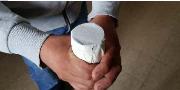
Figure 8. Tracing paper being placed in one extreme of the pipe.
